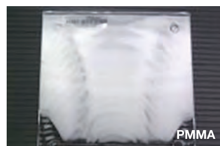
Ethanol solution Immersion Test (1 Day)
